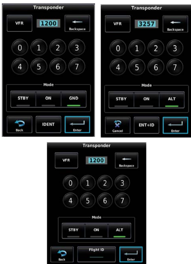
Transponder Code, Mode, and Flight ID Entry
