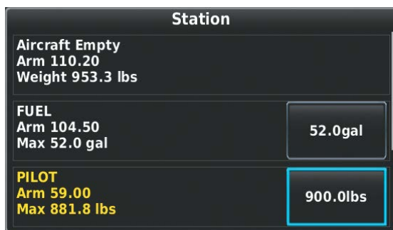
Loading Limit Exceeded
