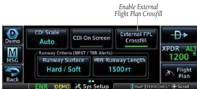
External Flight Plan Crossfill Enabled (Normal Mode)
