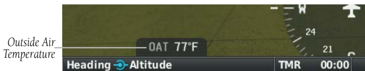
Outside Air Temperature on PFD (GDU 45X and GDU 470)
