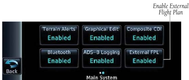
External Flight Plan Enabled (Configuration Mode)
