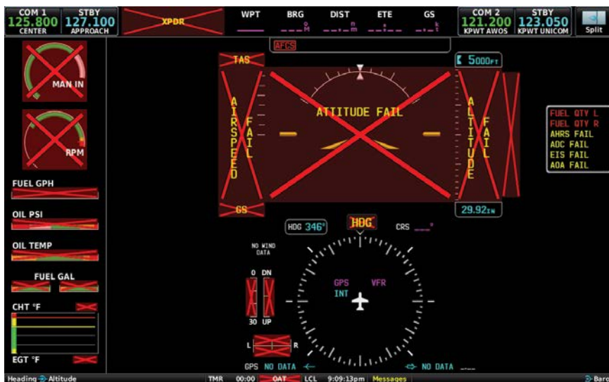
G3X Touch System Failure Annunciations
